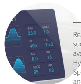
Real-time waveform, along with treatment data such as IPAP, EPAP, Vt, LK, MV and RR, etc. are available. The pulse oximeter can be connected to Hypnus PAP device wirelessly to show real-time SpO<sub>2</sub> and PR on ventilator screen. A comprehensive and professional therapy report can be generated.
